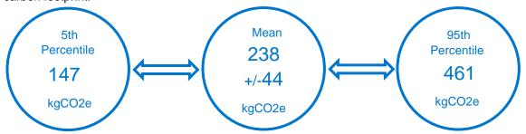
Carbon footprint calculations have a wide range based on a variety of factors including how the device is configured, where it was manufactured and more. Dell Technologies reports the 5th and 95th percentile of the carbon footprint estimate to reflect that uncertainty. For this product, that estimate has a mean of 238 kg of CO2e and standard deviation of 44 kg of CO2e.
