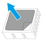
**c.** Install the heatsink on the controller.
